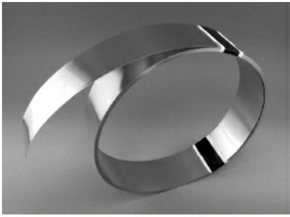
Solid copper strap (A) is the recommended material for grounding and bonding connection at RF. Flat-weave tinned braid (B) can be used if protected from water and corrosive gases or liquids. [Photos courtesy DX Engineering]
