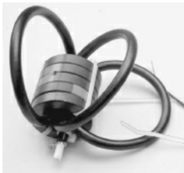
Figure 5.9 — (A) RF choke balun formed by coiling the feed line at the point of connection to the antenna. (B) Ferrite choke balun made by winding coax through a ferrite core. The chokes help isolate the outer surface of the feed line by blocking RF current. The ferrite choke is the preferred method of constructing feed line choke baluns.”
