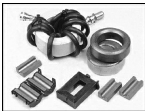
Figure 5.11 — A common-mode RF choke wound on a toroid core is shown at top left. Several styles of ferrite cores for common-mode chokes are also shown.
