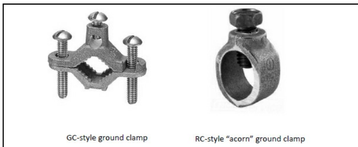
Figure 6.2 — Typical ground clamps. On the left is a type GC clamp used for making connections to pipe or tubing. An “acorn” or type RC clamp designed for ground rods is on the right.
