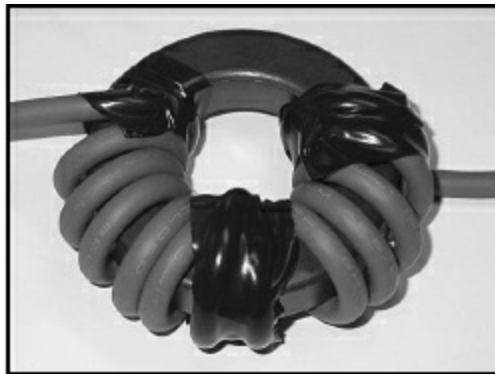
Figure 5.12 — A ferrite choke consisting of multiple turns of cable wound on a 2.4-inch OD toroid core.
