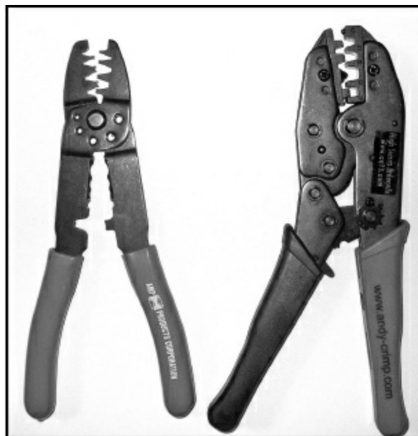
Figure 1.4 — Non-ratcheting (left) and ratcheting (right) crimping tool. The size of wires used for grounding and bonding requires the heavier tool to make a sturdy, reliable connection.
