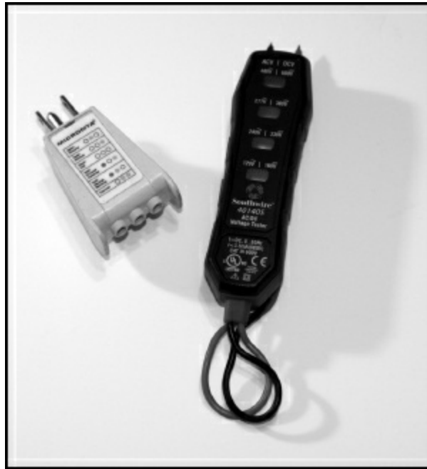
Figure 3.7 — Simple ac voltage tester (left) and plug-in ac circuit tester (right) for checking wiring. Always be sure a circuit is de-energized by using a tester.
